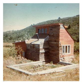
tamp it till it rings, hard packed. Keep adding earth-mix, keep tamping, and the walls rise. With a "hat and shoes" - protective roof and foundation - a
